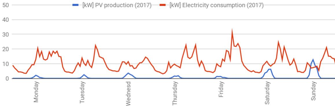
Figure 5. Actual production and consumption data logged by the PV inverters during one week in December, 2017.
